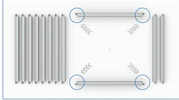
4 Bridge the two parallel bottom frame lengths to make a square base
