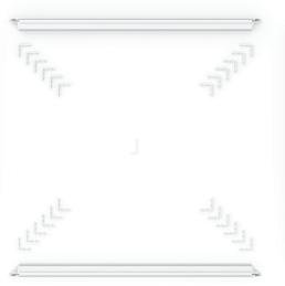
2 Insert corner bracket into frame length (ensuring the bracket is set in as far as possible)
